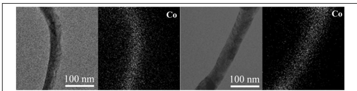
Fig. 7. TEM images of (a) as-implanted and (c) high-vacuum annealed  $Zn_{1-x}Co_xO$  NWs with a dose of  $6 \times 10^{16} \text{ cm}^{-2}$  and an average diameter of 38 nm. EDX mapping images of the Co element in (b) as-implanted and (d) high-vacuum annealed  $Zn_{1-x}Co_xO$  NWs.
