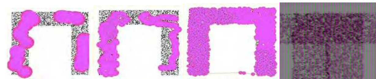
Fig. 19. Identification of patterns with ParaSOM: a) network at 100 iterations; b) network state at 400 iterations; c) 600 iterations; d) in spite of the input distribution, the single object is identified
