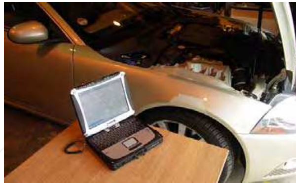
Fig. 9. Diagnostic tool for reading DTCs.
