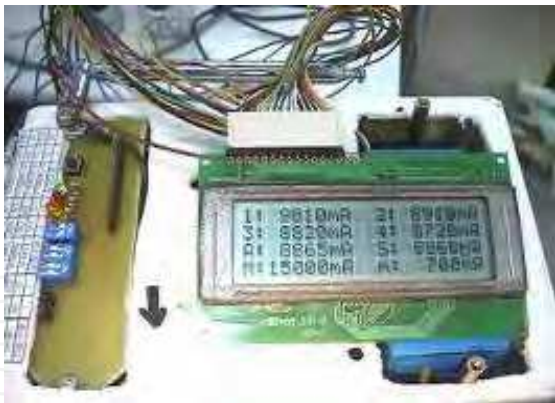
Fig. 4. The prototype of the power detection module
