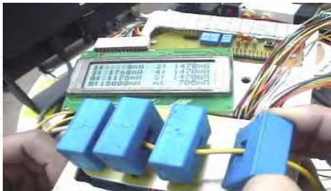
Fig. 12. The current sensor #1 and #3 are wrong
