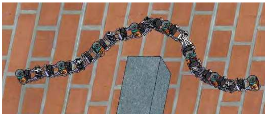
Fig. 3. 3D-animation of the planned robotic caterpillar
