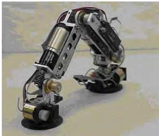
Fig. 3. RAMR1 biped climbing robot (Tummala et al. (2002))
