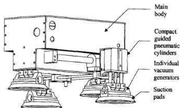
Fig. 1. ROBICEN III climbing robot (Savall et al. (1999))
