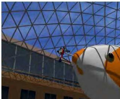
Fig. 19. Balloon-based robot consisting of a walking mechanism and a cleaning tool (Elkman et al. (2002))
